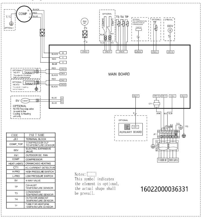
Outdoor unit printed circuit board diagram: 17122000047115
